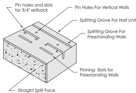
**Standard Wall** can be used to build retaining walls, freestanding walls, columns, privacy fences and outdoor living features.
